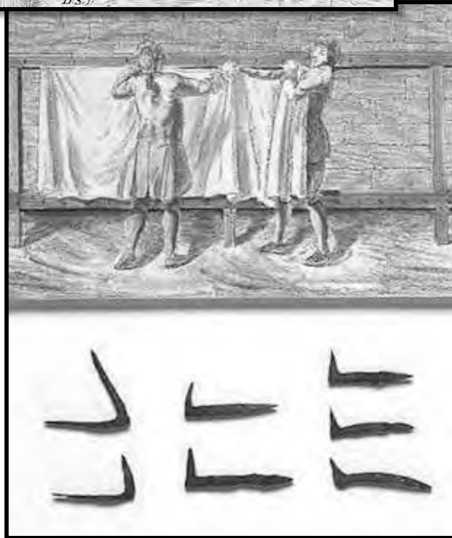
Image top: Fulling Mill Mechanism. Image above: Fulfilled fabric being stretched on tenter hooks
